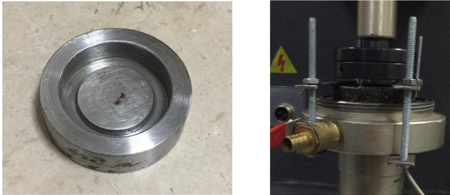
Figure 27: (a) mould for sample preparation (b) test assembly for friction coefficient test
