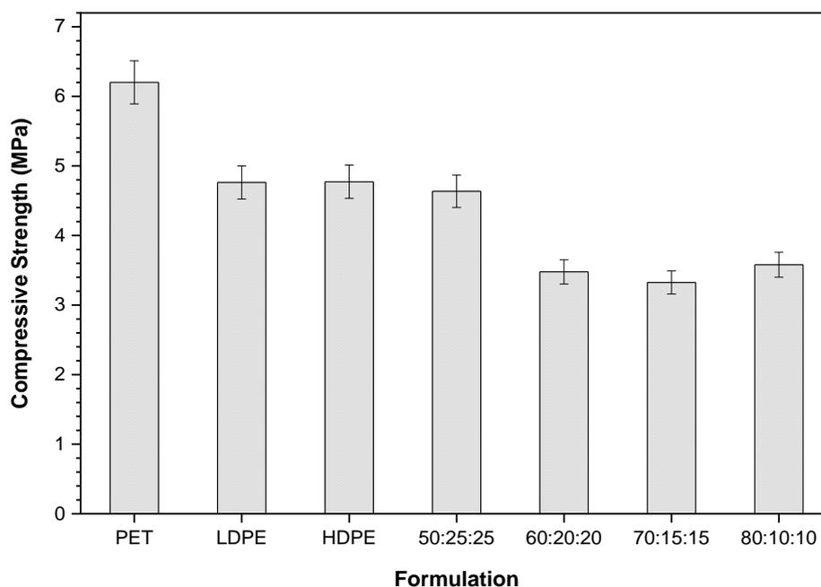
Figure 5: Compressive strength of different dosages of waste plastic to be used in manufacturing of waste plastic brick
