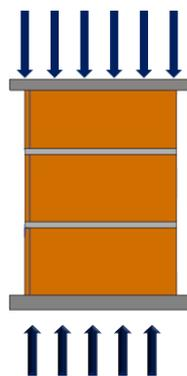
Figure 34: Schematic diagram illustrating the compressive test for brick prism
