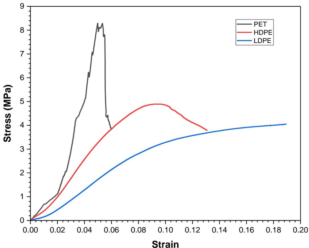
Figure 6: Stress strain plot of PET, HDPE & LDPE
