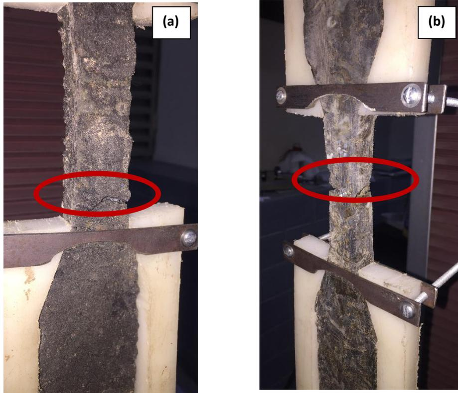
Figure 33: Failure of specimens under tension (a) 50:50 (b) 100:0
