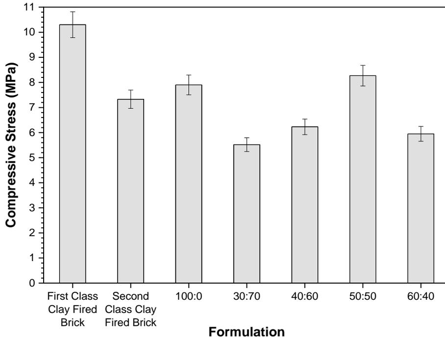
Figure 8: Compressive strength test for control and waste plastic brick formulations
