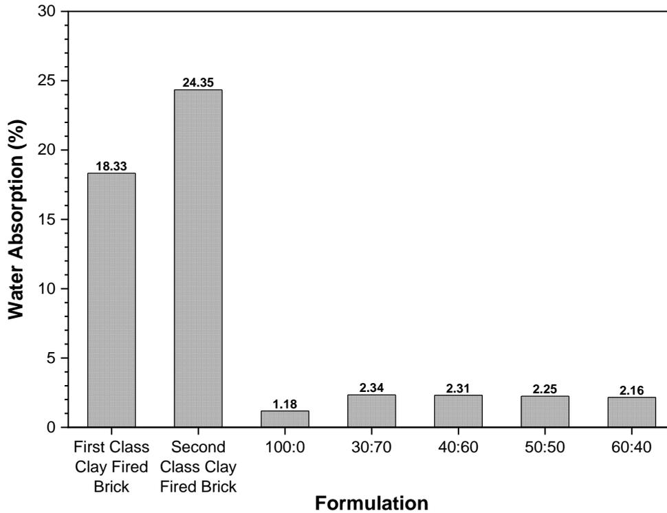
Figure 11: Water absorption for different formulations of control and waste plastic brick
