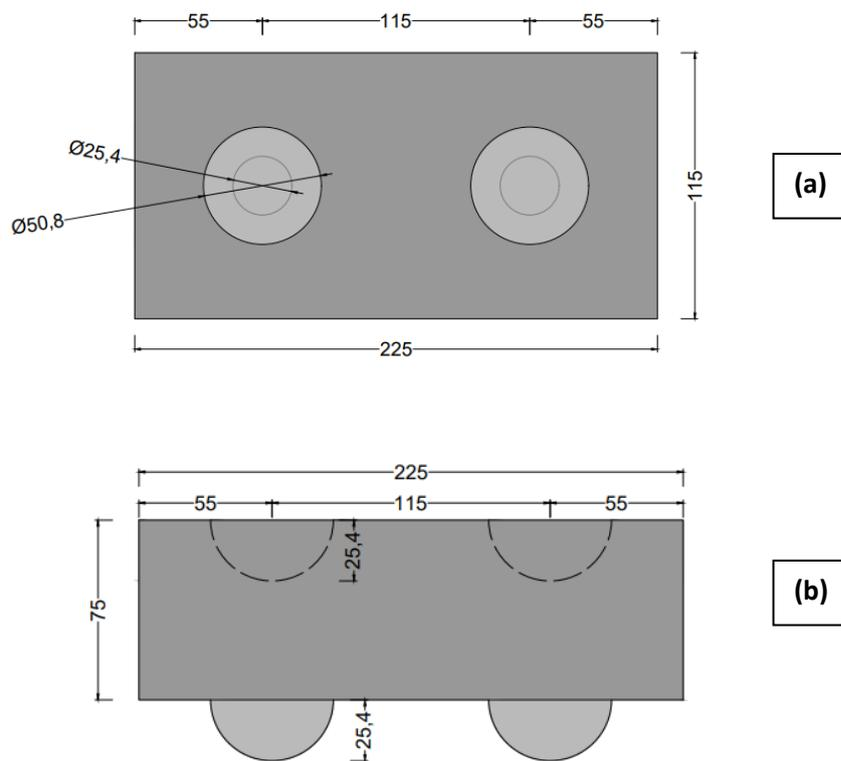
Figure 37: Dimensions of waste plastic interlocking brick (a) plan view (b) side view
