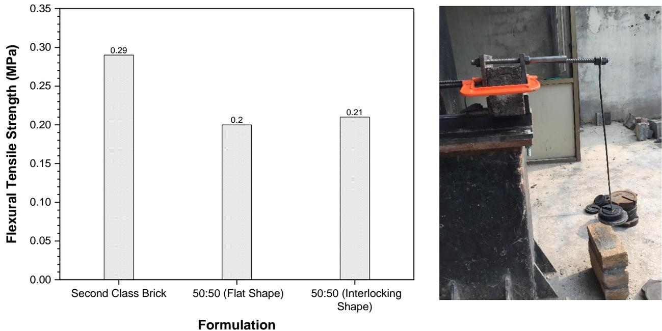
*Figure 18: Flexural Tensile Strength of second class brick, waste plastic brick 50:50 flat shape and interlocking shape*
