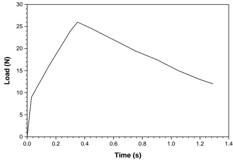
Figure 29: Load versus time plot for friction coefficient test
