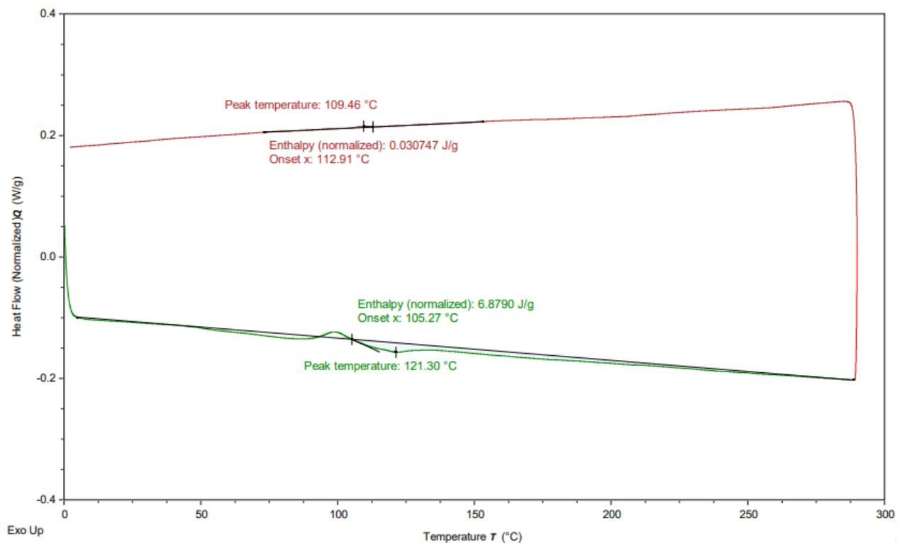
Figure 23: DSC of waste plastic brick formulation 50:50
