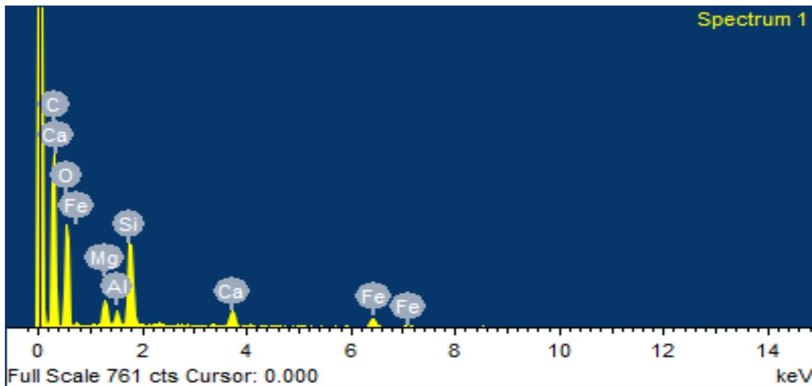
Figure 21: EDS spectrum of waste plastic brick formulation 50:50
