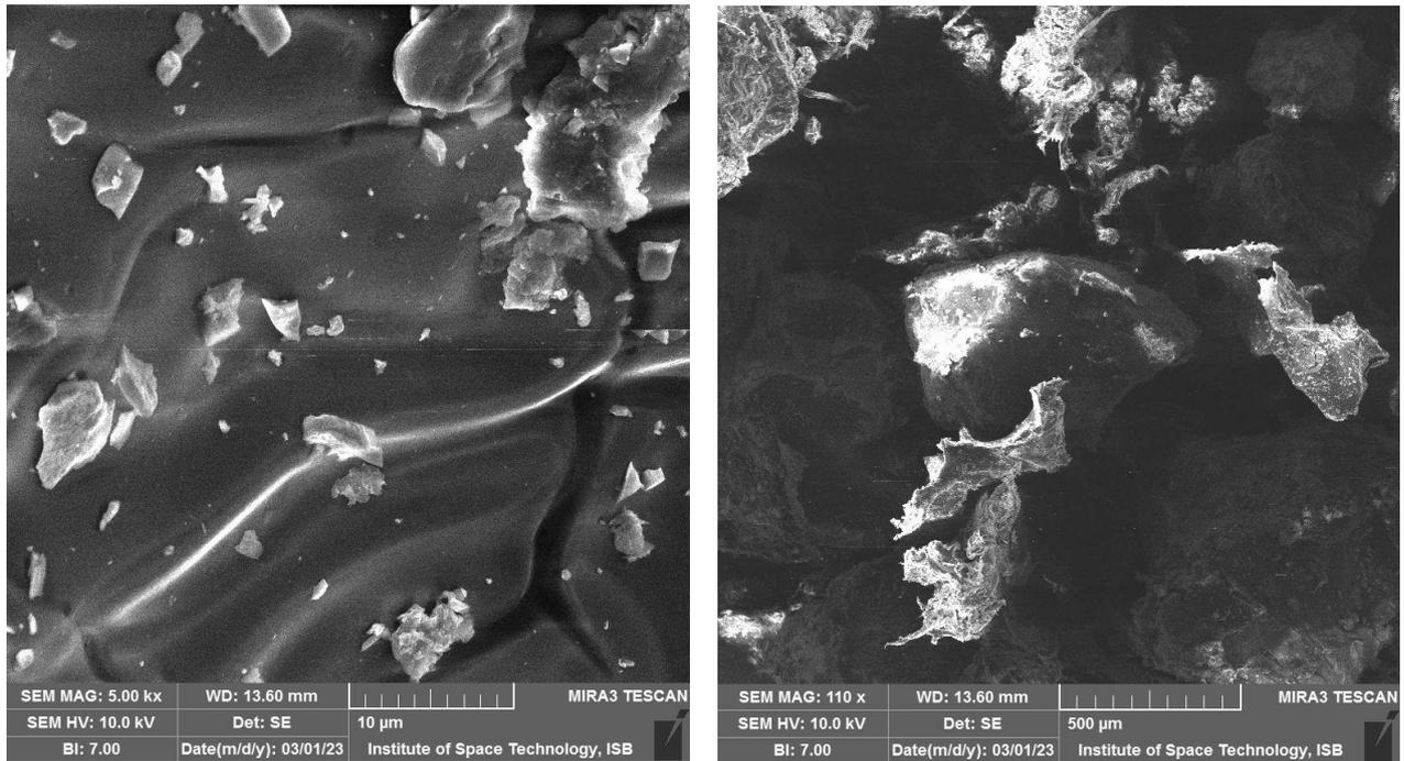
Figure 19: SEM image of waste plastic brick formulation 50:50
