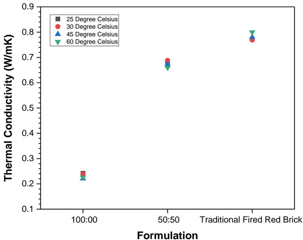
Figure 22: Thermal conductivity for different brick formulations
