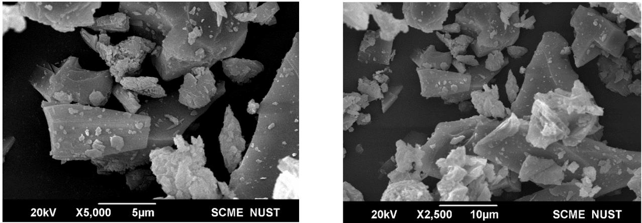
Figure 2: SEM of WFS highlighting particle morphology
