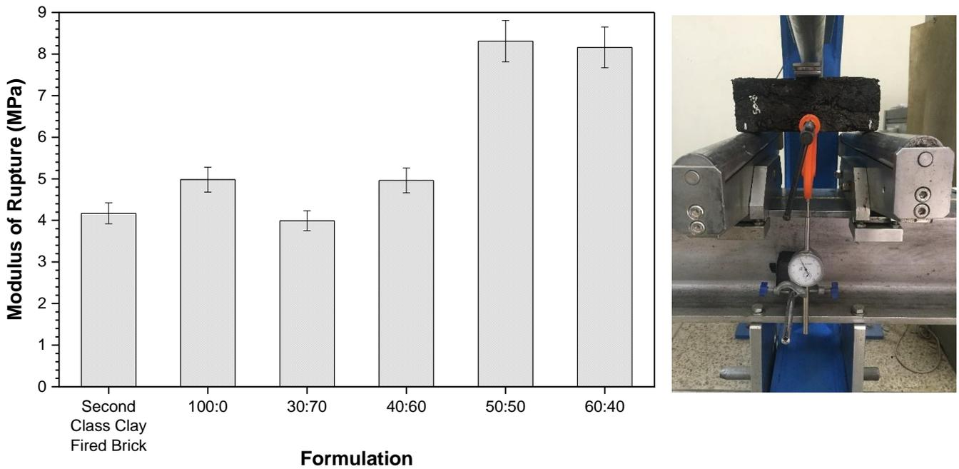
Figure 15: Modulus of rupture for control and different waste plastic brick formulations
