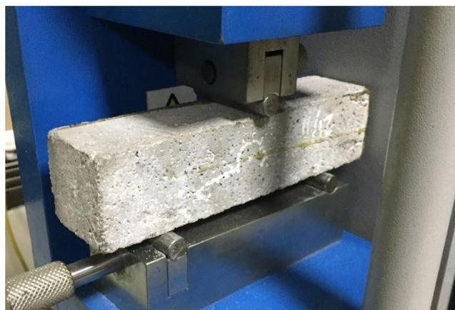
*Figure 26: Flexural test on mortar prism*
