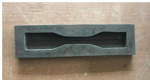
Figure 30: Mould prepared for casting of tensile specimens
