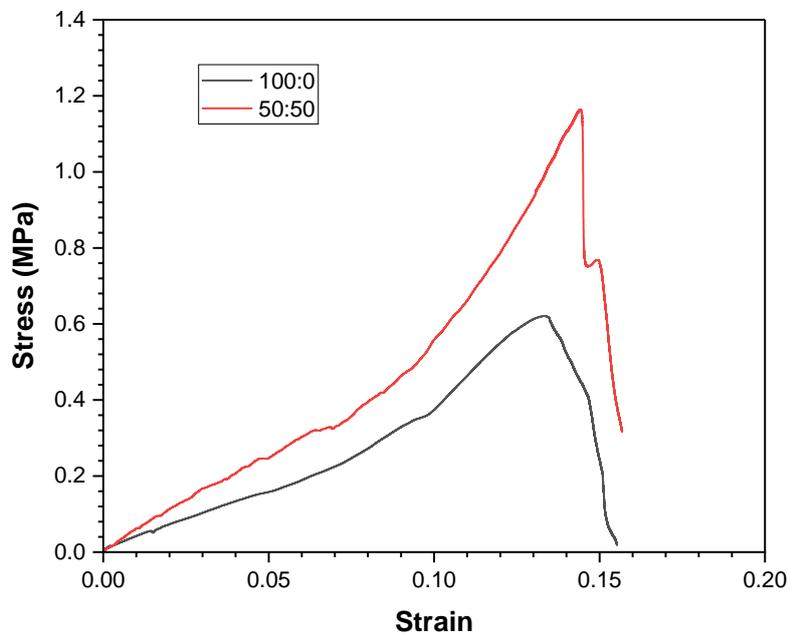
Figure 32: Stress strain plot for tensile strength of the specimens
