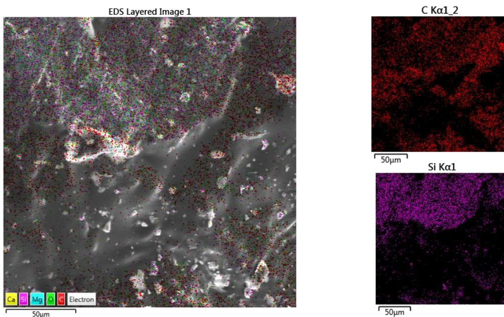
Figure 20: EDS mapping of waste plastic brick 50:50
