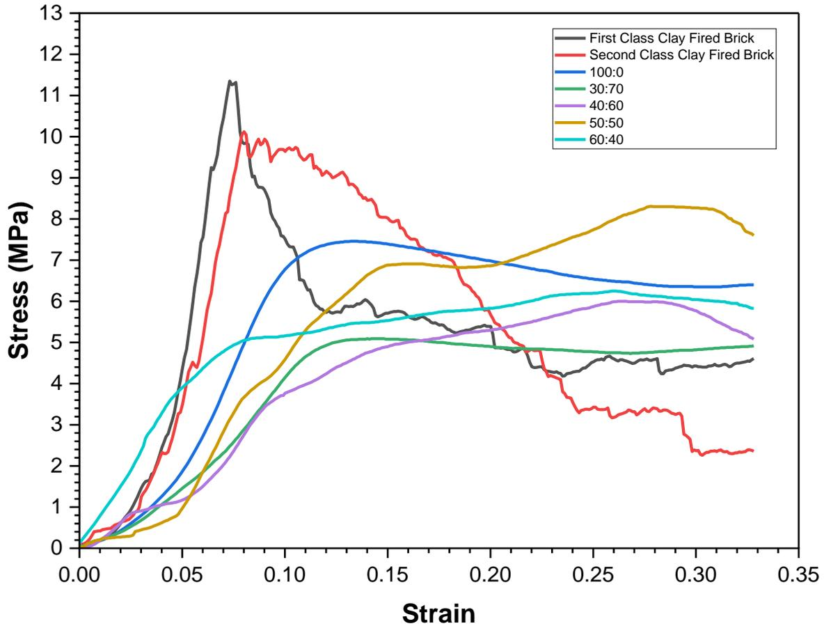
Figure 10: Stress strain of various formulations of control and waste plastic brick
