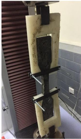
Figure 31: (a) Dimension of prepared sample (b) sample mounted on tensile testing machine
