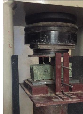
Figure 17: Splitting tensile strength of control and waste plastic brick formulations
