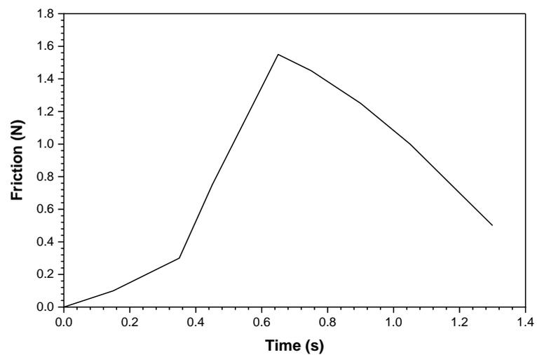
Figure 28: Friction versus time plot for friction coefficient test
