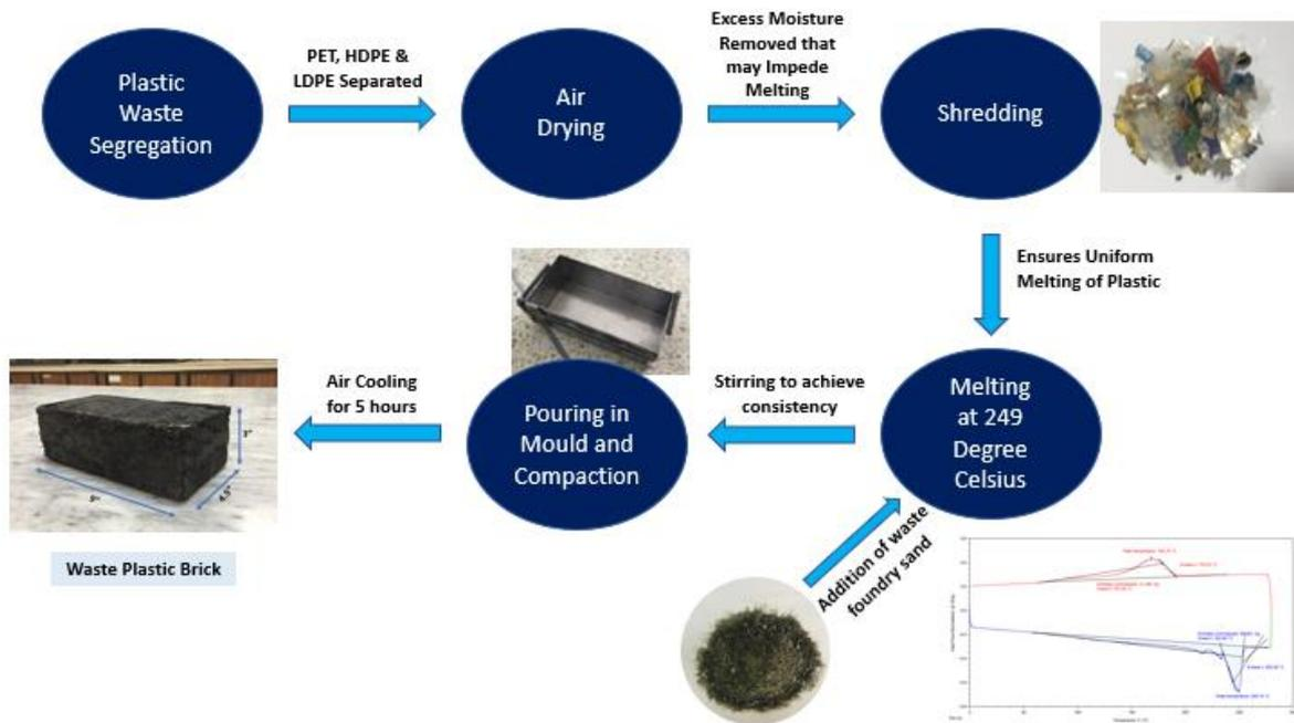
Figure 4: Schematic diagram illustrating the casting procedure of waste plastic brick
