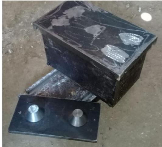
Figure 36: Moulds used for casting waste plastic interlocking brick
