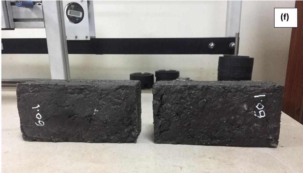
Figure 13: Efflorescence test results for (a) second class brick (b) 100:0 (c) 30:70 (d) 40:60 (e) 50:50 (f) 60:40
