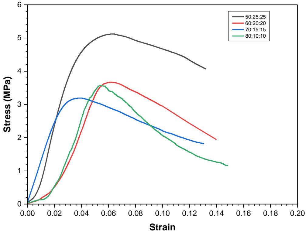
Figure 7: Stress Strain plot for various PET/HDPE/LDPE blends
