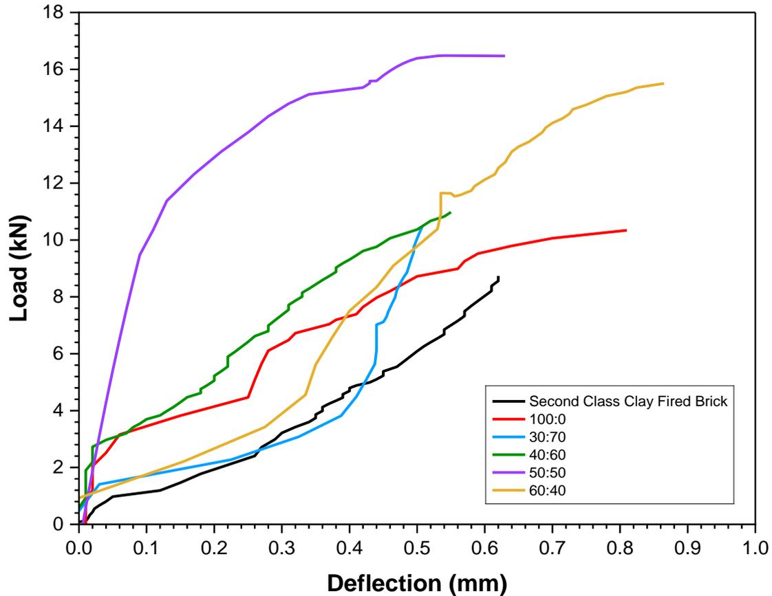
Figure 16: load deflection curves for control and waste plastic brick formulations
