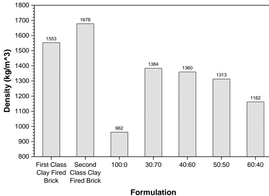
Figure 14: Density for control and different waste plastic brick formulations
