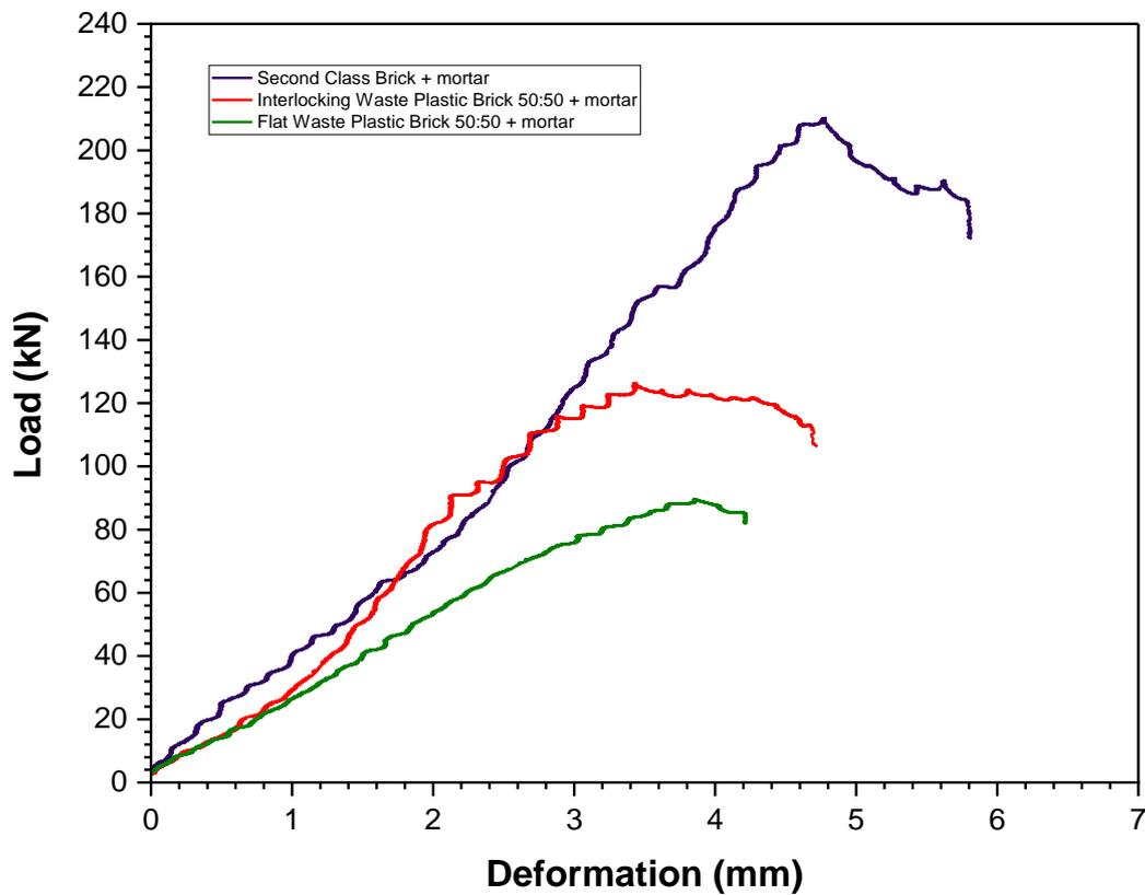
*Figure 35: Load deflection curve for various brick formulations*
