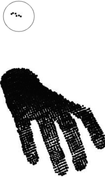
Figure 3.1: Hand Point Cloud generated from Single View (Before DBSCAN)
