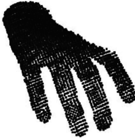
Figure 3.2: Hand Point Cloud generated from Single View (After DBSCAN)
