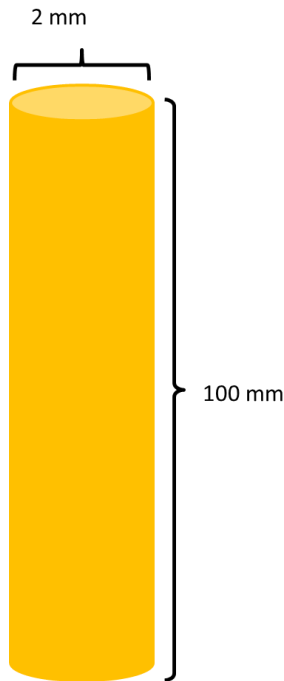
Figure 3.6: Specifications of Test Sample- Shape Memory Alloy
