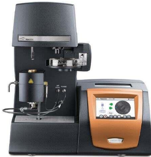
Figure 5.2. TGA instrument (TA TGA5500)
