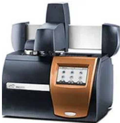
Figure 5.1. DSC instrument (TA DSC250)
