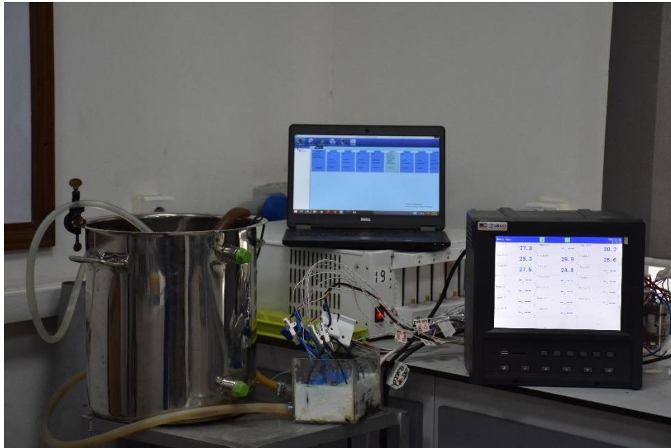
Figure 3.6. Experimental system of hybrid cooling of Li-ion battery pack
