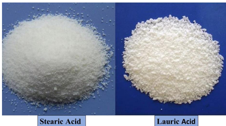
Figure 3.5. Stearic acid and Lauric Acid PCM
