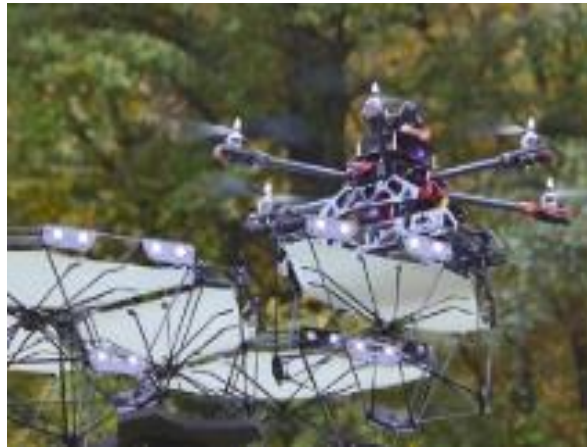
Figure 2.8: UAVs being used to assemble a simple fibre structure using custom-made lightweight material (Wood et al., 2019).
