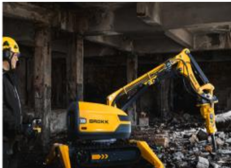
Figure 2.4: A teleoperated heavy equipment with a jackhammer attached developed by BROKK (Melenbrink et al., 2020).
