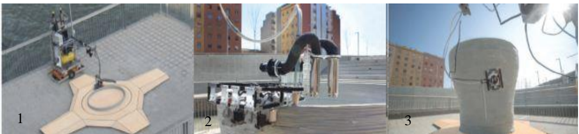
Figure 2.9: The Mini-builders project using 3 distinct but collaborating task-specific robots to construct a ceramic structure (Jokic et al., 2014).
