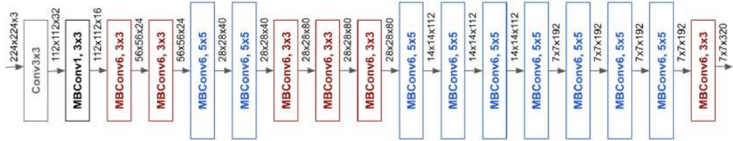
Figure 5.3: Mobile inverted convolutional layers form the bulk of the EfficientNet B0. Image taken from [11]
