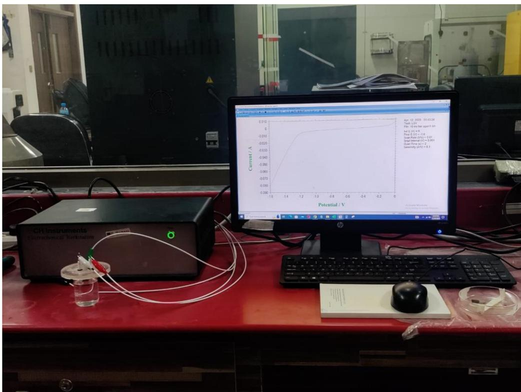
**Figure 3.3: Electrochemical workstation setup**
