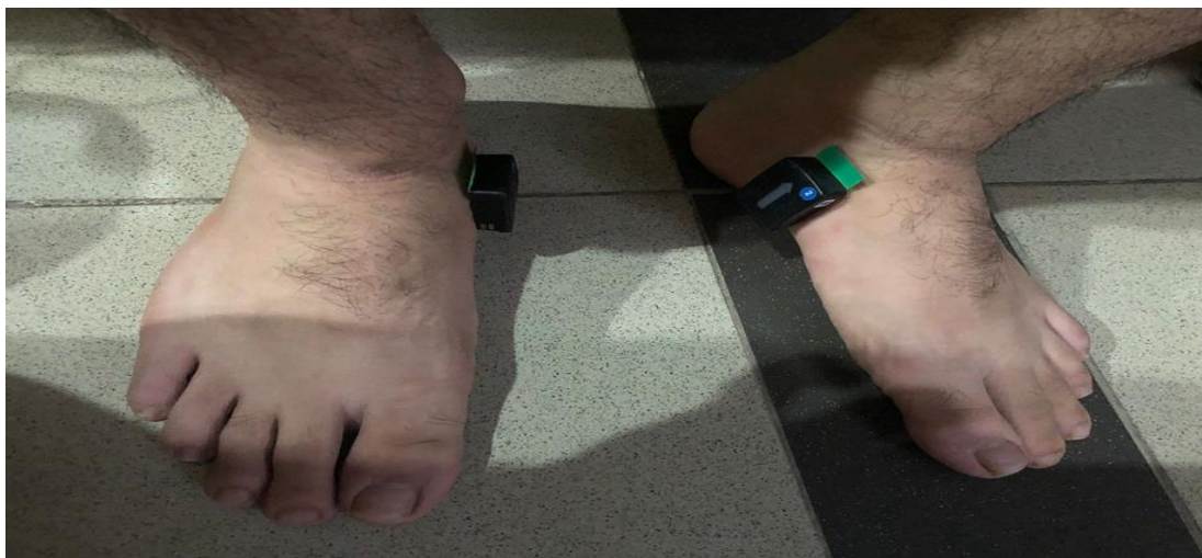
Figure 12: The placement of the Delsys Trigno Avanti Sensor is shown on the first cunieform.
