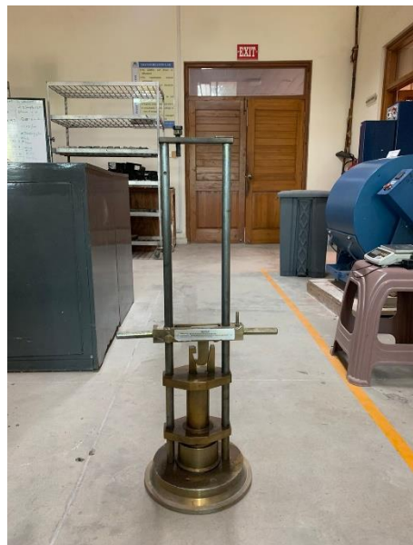
Figure 3.4 aggregate impact value test
