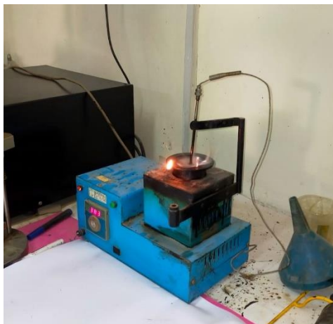
Figure 3.9 flash and fire point test
