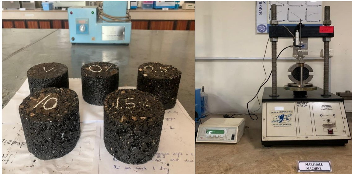
Figure 3.18 Indirect Tensile Strength (IDT) and Moisture Susceptibility Testing
