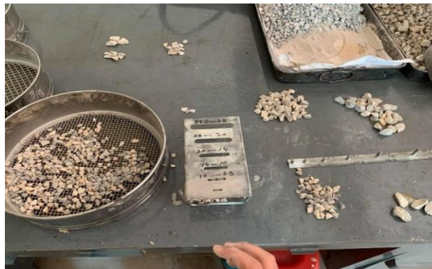
Figure 3.5 Flakiness & Elongation Test
