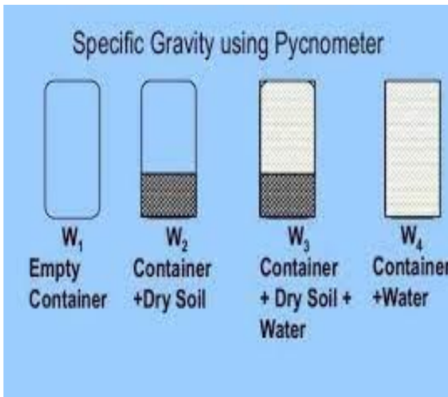
Figure 3.6 Specific Gravity Test
