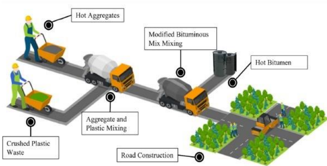
Figure 3.23 Dry Mixing Process
