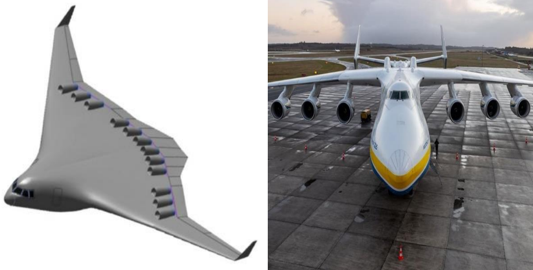
Figure 2.5 Distributed discrete fan in blended wing body and podded engines
