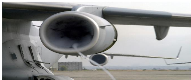
Figure 2.12 Tightly vortex generated in Podded engine.
