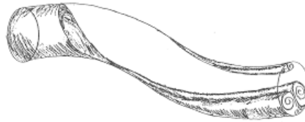
Figure 2.11 Paired swirl in S-duct
