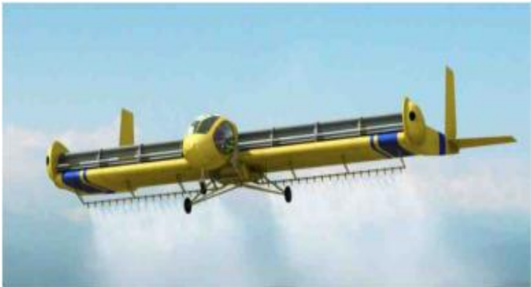
Figure 2.4 Cross flow fan application in aircraft
