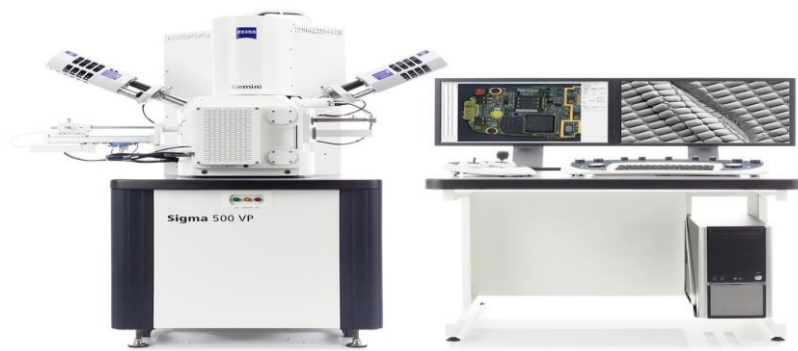
Figure 10: Scanning Electron Microscope (ZEISS Sigma 500 VP, NCP)
