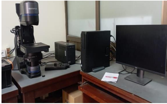
Figure 8 & 9: Olympus Corporation DSX1000 UZH Digital Microscope
