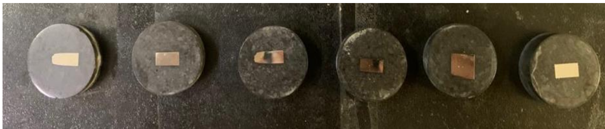
Figure 11: Original Samples after EDM wire cut.
