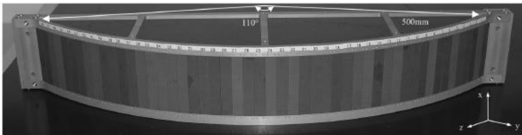
Figure 3.52 Prototype conformal phased array antenna [23]
