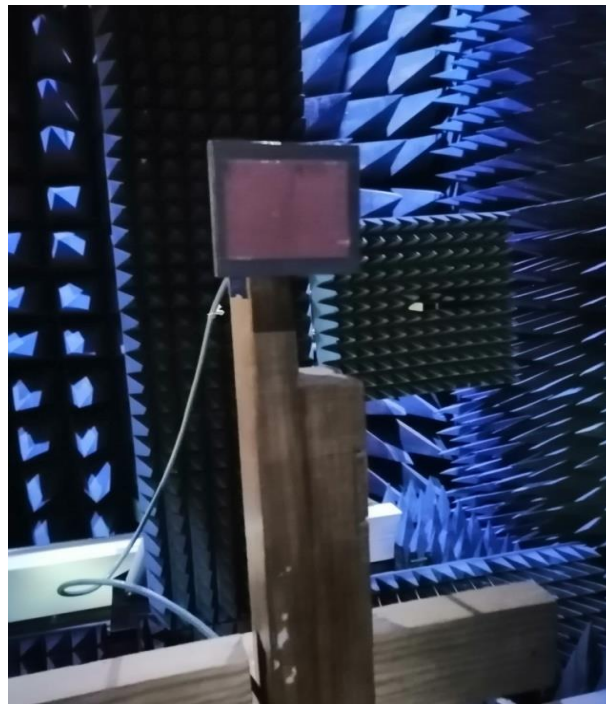
Figure 4.83 Antenna placed in the anechoic chamber
