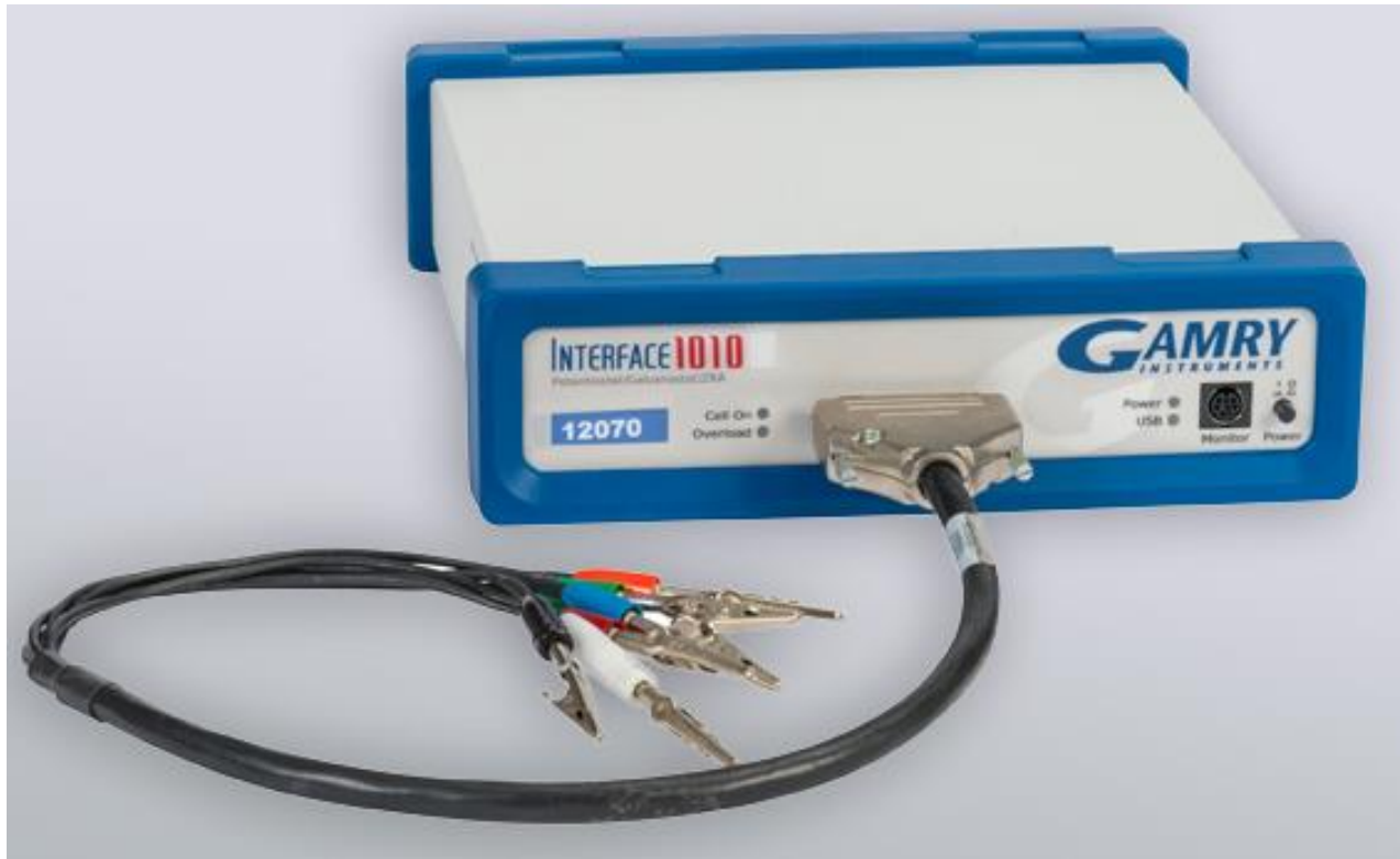
Figure 10. Potentiostat interface instrument through which the EIS and potentiodynamic polarization measurements can be measured [31]
