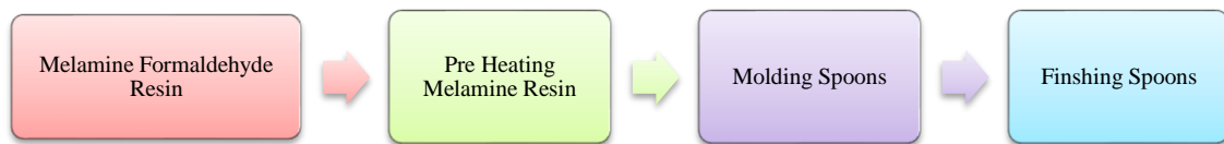
Figure 1.1: Melamine cutlery manufacturing process.
