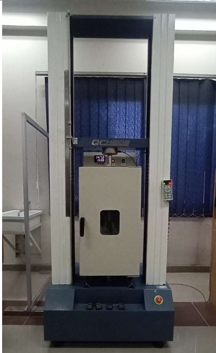
Figure 3.4: Haida HD B607-S Universal Testing Machine with Thermal Chamber.
