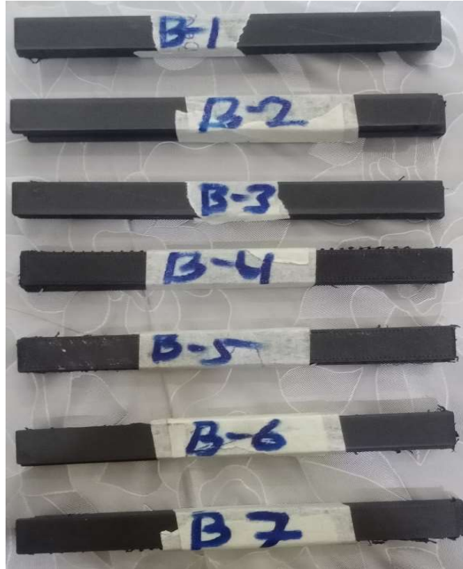
Figure 3.3: 3D Printed Onyx and HSHT Glass fiber composite specimens.
