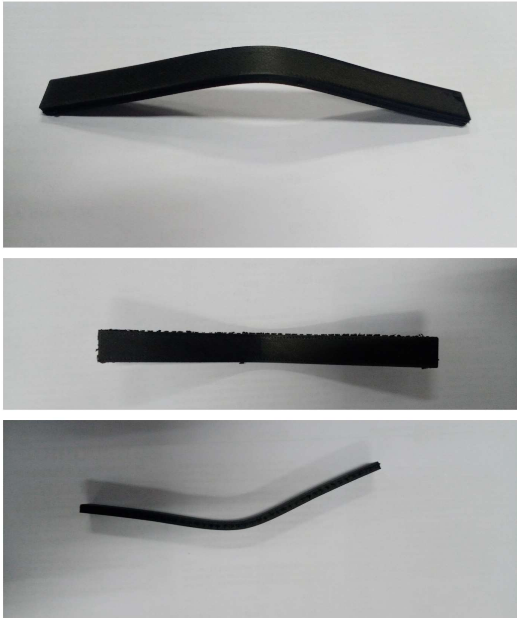
Figure 4.2: Composite test specimen after undergoing flexural test.
