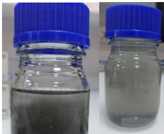
Figure 3.5: Supernatant After first and second centrifugation.
