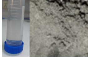
Figure 3.8: 2D TiB 2 solution in supernatant After centrifugation and Dried 2D TiB 2 sheets.
