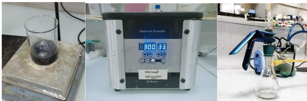
Figure 3.4: Magnetic Stirring Hotplate, Centrifuge and Vacuum Filtration Assembly used in the experimentation.
