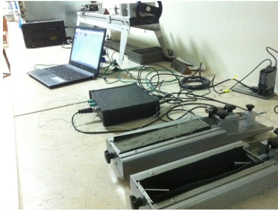
Figure 3.11: Modified German Shwindrine Shrinkage Apparatus
