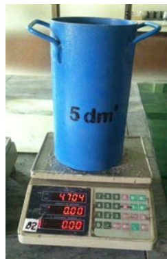
Figure 3.6: Container used for determining packing density
