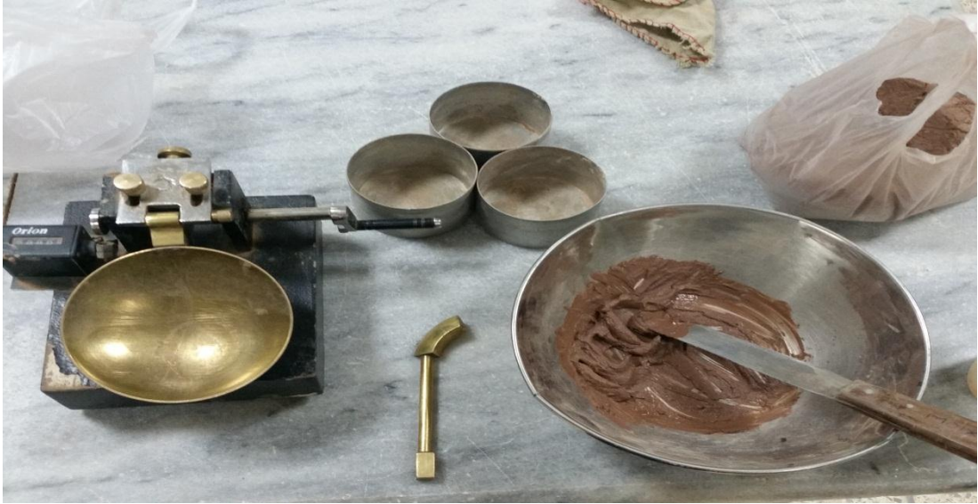
Figure 3. 4: Casagrande's apparatus for finding Liquid Limit of Soil
