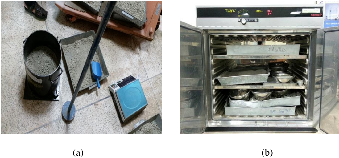
Figure 3. 2: (a). Pulverizing sun dried soil sample (b). Oven drying soil sample at 105 degree Celsius
