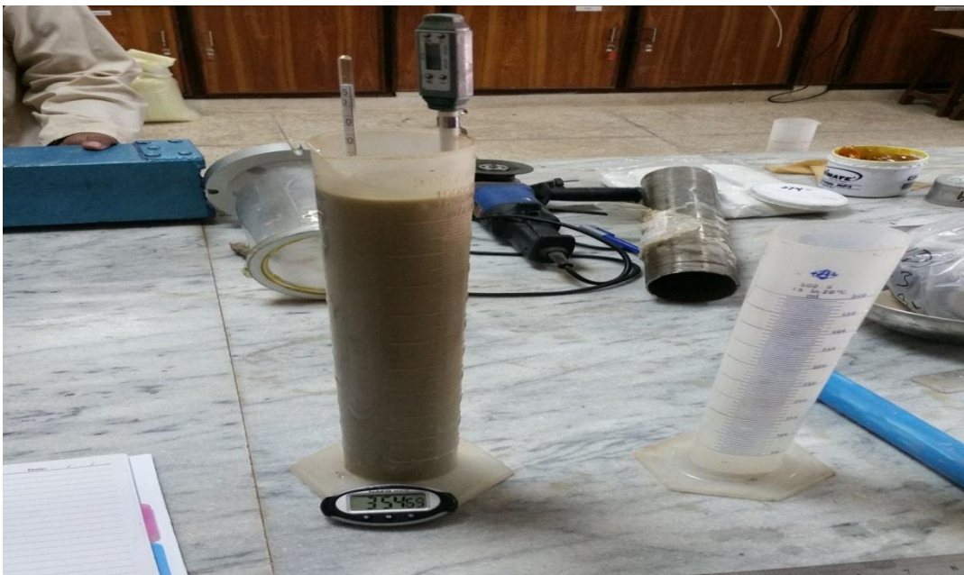
Figure 3. 3: Hydrometer Analysis of Soil sample
