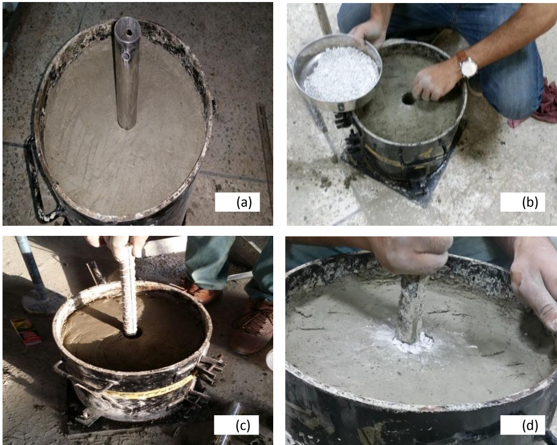
Figure 3. 13: (a) Removal of soil by replacement method (b) Pouring of crushed stone from top (c) Compaction of crushed stone to required density (d) Stone column in soil sample
