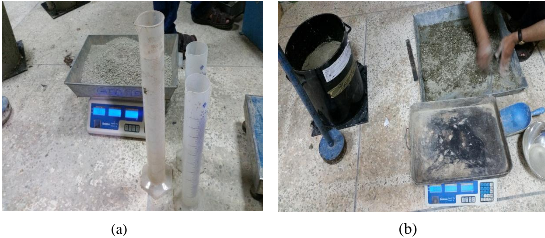
Figure 3. 10: (a) Calculating amount of soil and water (b) Mixing of soil and water for clay bed
