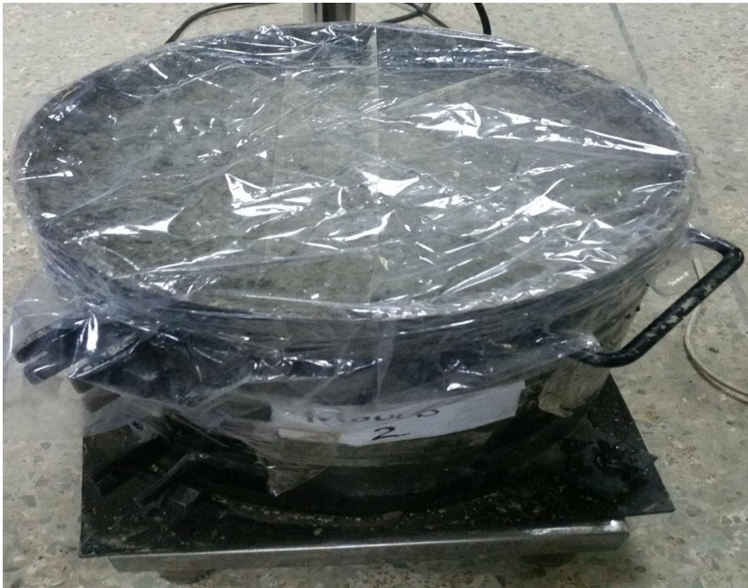
Figure 3. 12: Compacted soil bed covered in polythene sheet for uniform transfer of moisture
