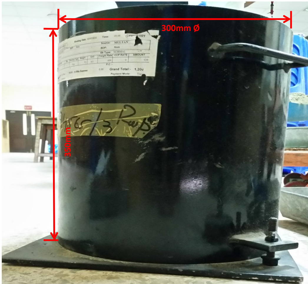
Figure 3. 9: Special steel mold for Load testing of soil (Not to Scale)
