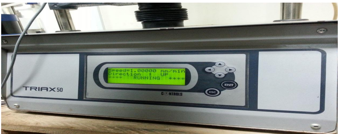
Figure 3. 7: Control Unit of TRIAX50 Tri-Axial Compression Test machine
