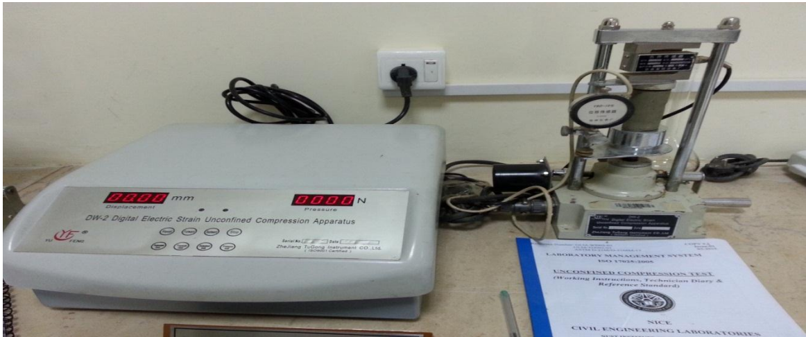
Figure 3. 6: Unconfined Compression Strength test using digital electronic strain UC apparatus
