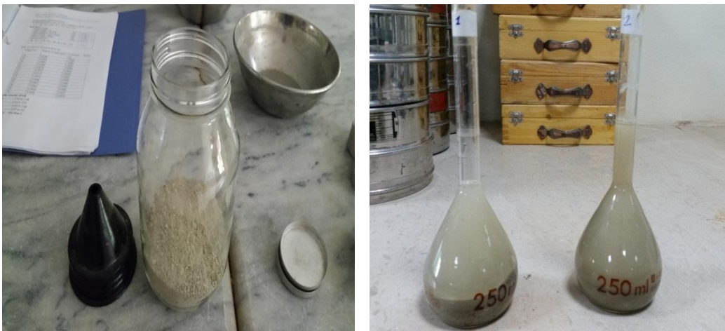
Figure 3. 5: Performing Specific Gravity test using (a) Pycnometer and (b) Volumetric flasks
