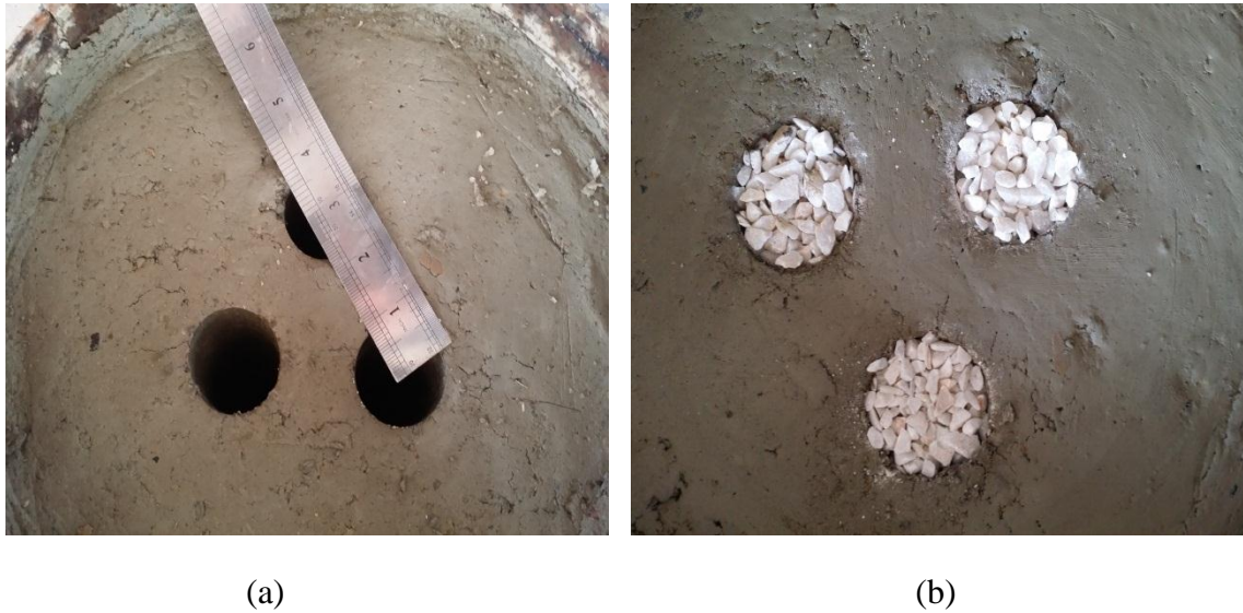
Figure 3. 14: (a) laying out triangular arrangement for stone columns (b) 3 stone columns in triangular arrangement
