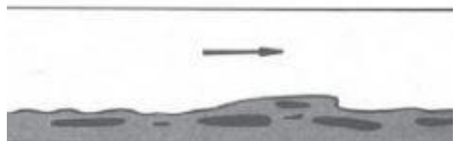
Figure 2.3: Stratified three-phase flow patterns of Gas-Liquid-Liquid [47]
