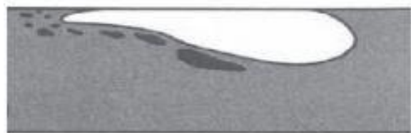
Figure 2.5: Slug three-phase flow patterns of Gas-Liquid-Liquid [47]
