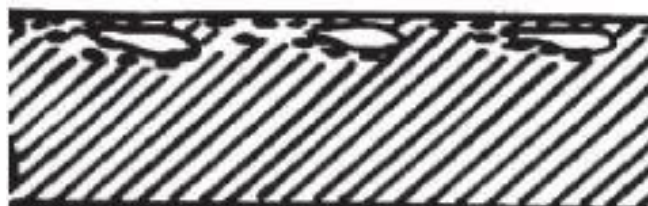
Figure 2.4: Plug three-phase flow patterns of Gas-Liquid-Liquid [47]
