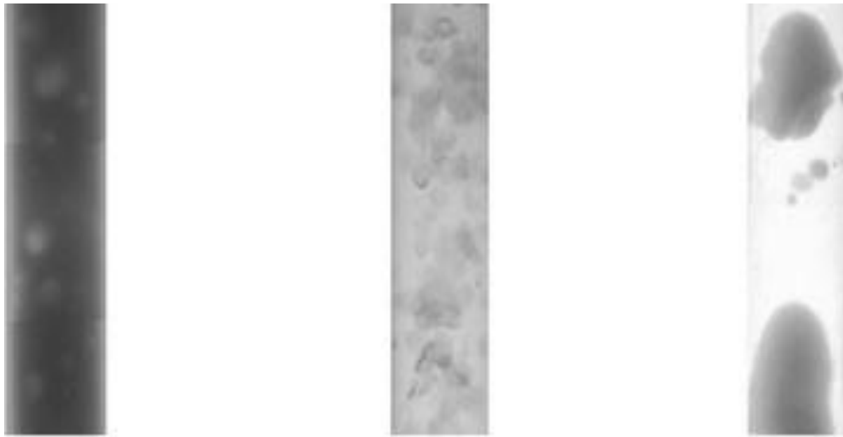
a) Bubbly oil-based flow
