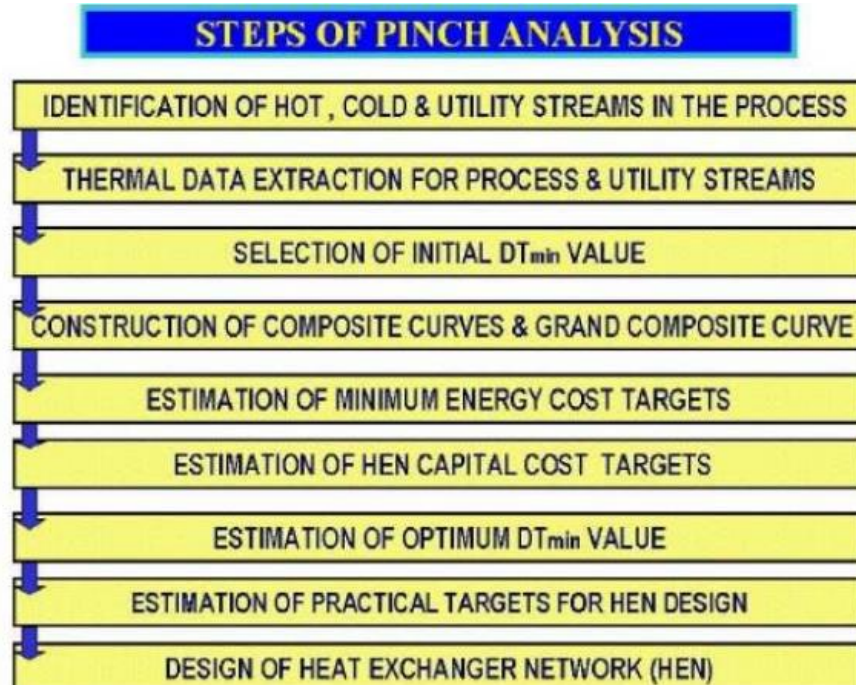
Figure 4-1 Steps Of Pinch Analysis
