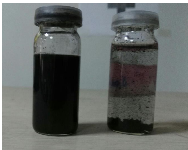
Figure 0-13 Dispersion of functionalized and pristine CNTs at left and right respectively
