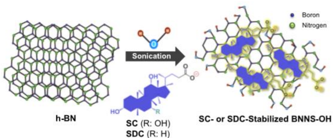
Figure 2-9: Schematic diagram of noncovalent functionalized BNNS-OH [47]
