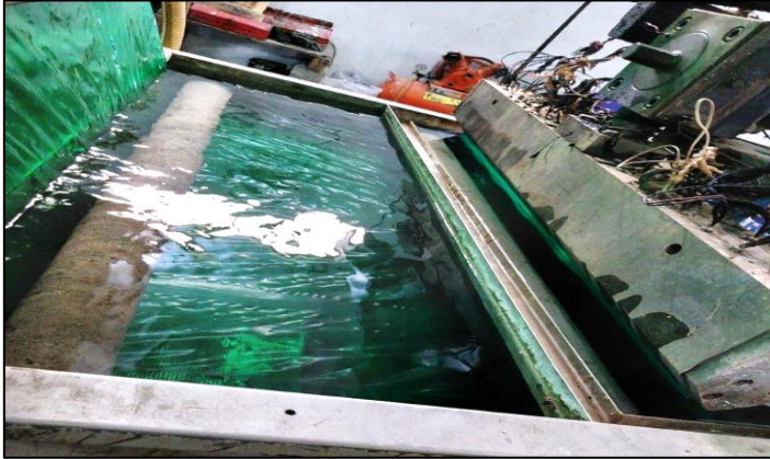
Figure E4: Conversions to yarn through dies and cooling in cool water tank.
