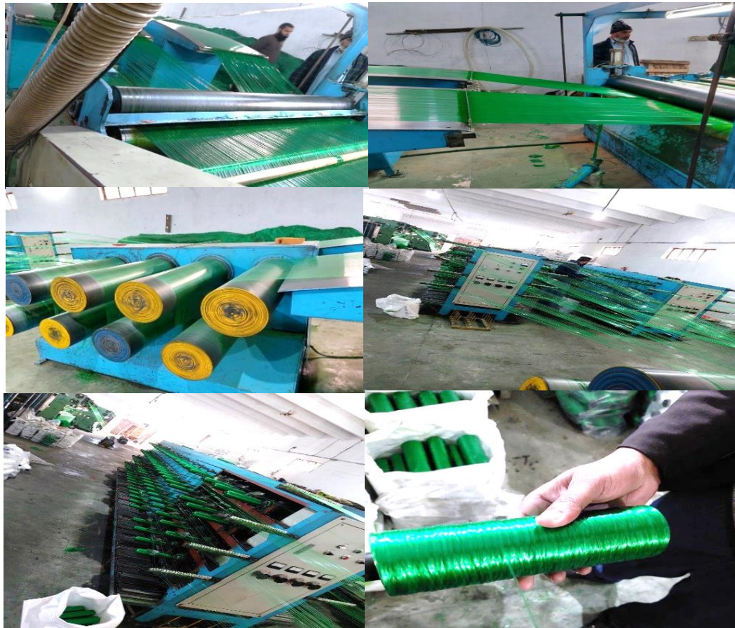
Figure E7: Cutting and Winding on beams and bobbins
