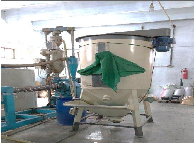
Figure E2: Automatic Mixing through Hopper
