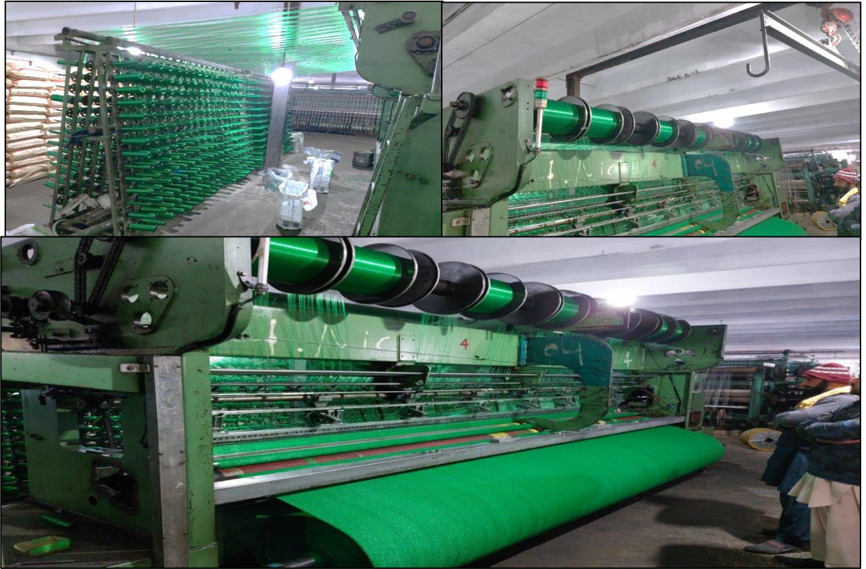
Figure F1: Knitting of Greenhouse Shade Cloth on Raschel Knitting Machine
