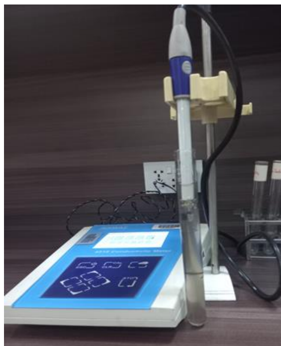
Figure 5. 10 Set up for ionic Conductivity Measurement
