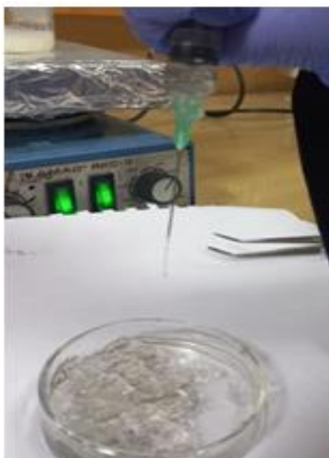
Figure 5. 6 Setup for Injectability measurement of hydrogels
