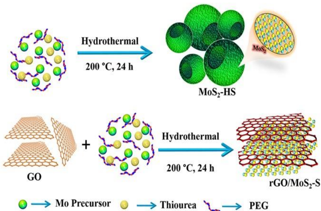
Figure 1.5 Schematic of MoS 2 /rGO for energy conversion and storage application
