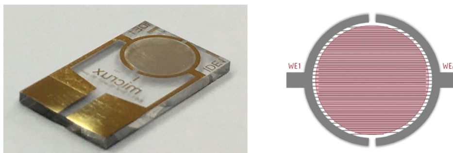
Figure 3: Typical structure of a Gold IDE (a) with enlarged working area (b).
