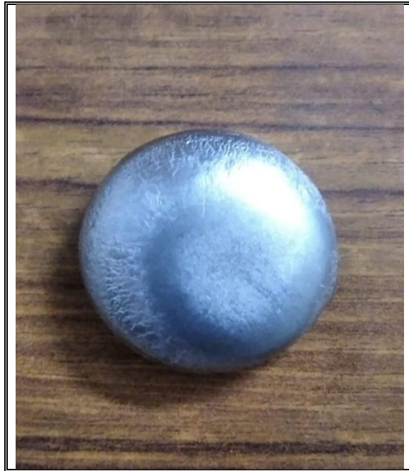
Figure 13: Button shape metallic sample produced from arc suction melting furnace. EDM wire cut then cut the metallic buttons into desired shapes to perform further characterization.
