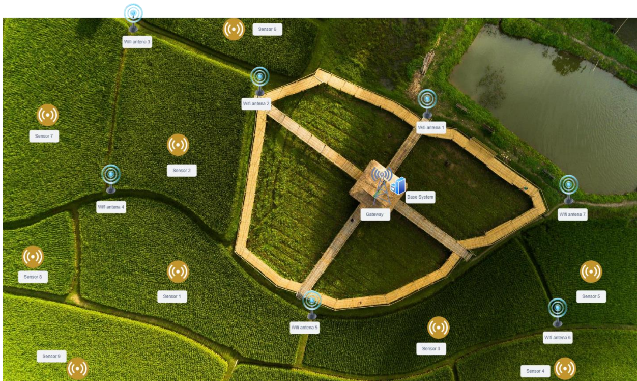
Figure 5.1: Overview of IoT Network for Monitoring
