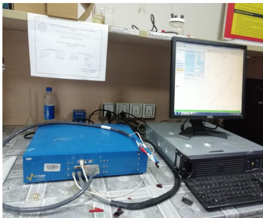
Figure 11 EC workstation in surface lab of SCME (NUST) Islamabad, which is used for measuring CV for our IL based SC.
