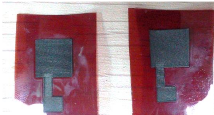
Figure 6(a) Laser software on computer with electrode drawn on it (b) Laser scribed PI sheet with 1x1cm electrode's dimension and connecting electrodes
