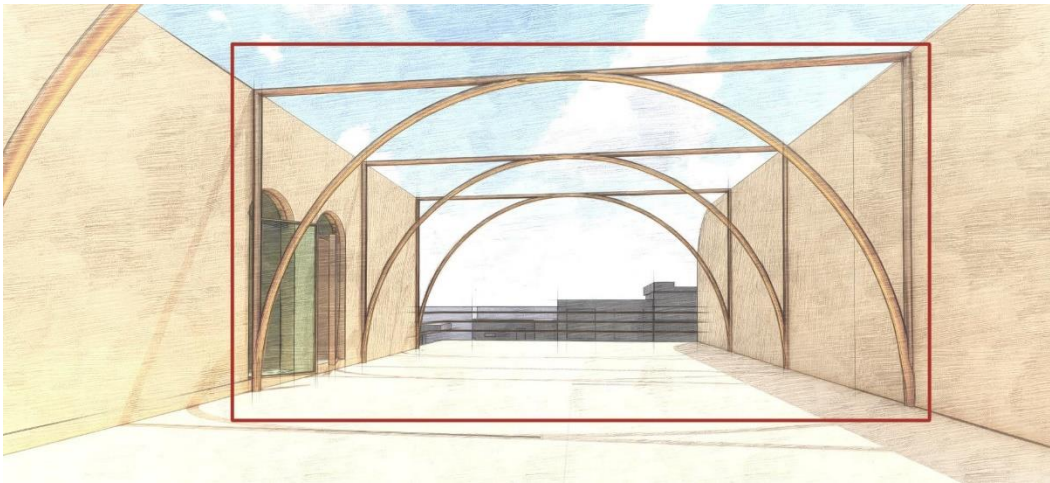
Figure 0.5 Materiality changes. The same arch design as on ground floor, with a lightweight, more processed material. Used for ornamentation. Source: Author
