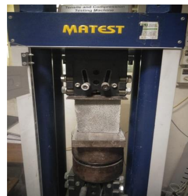
b) Compression test setup
