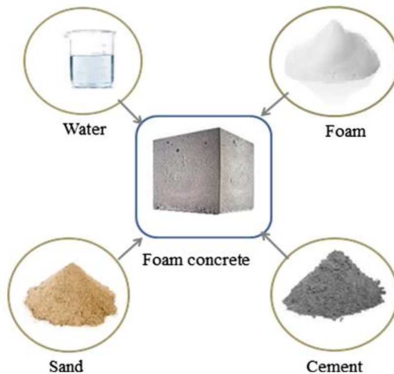
Figure 2.3 Materials for Cellular Lightweight Concrete [12]
