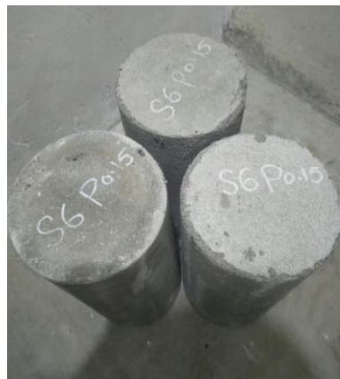
Figure 3.4 Split Tensile Strength Testing
