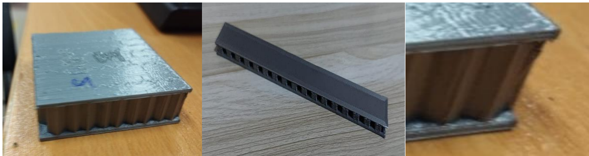
Figure 10: Printed Honeycomb Samples illustrating no any prominent printing defect. No any Stringing, curling and weak infill observed.
