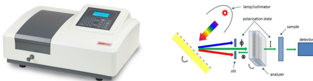
Figure 3.2: UV spectrophotometer and its working principle
