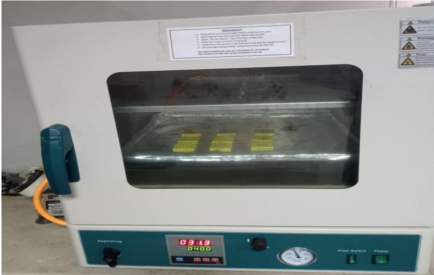
Figure 4.2: Drying sample using vacuum furnace.
