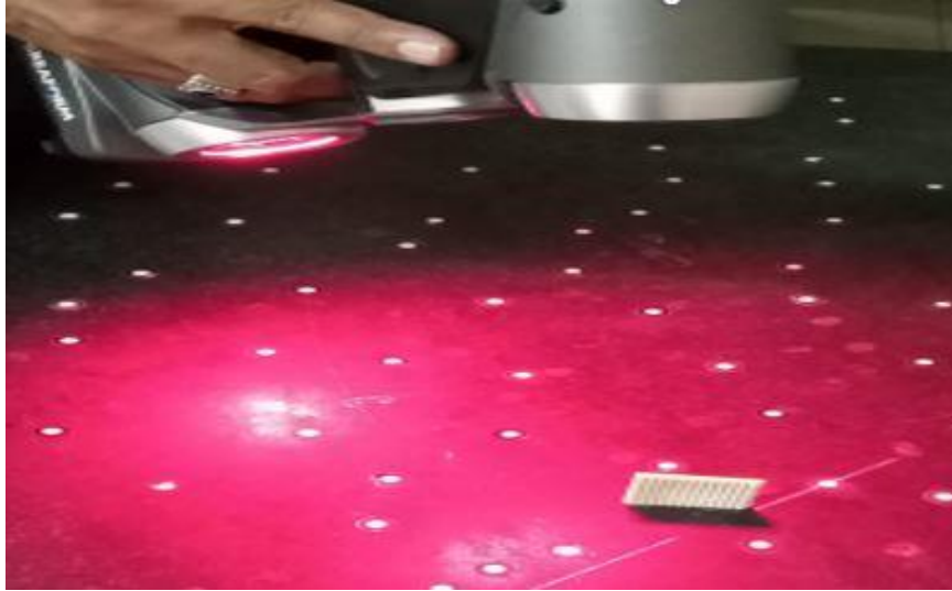
Figure 3.8: Scanning samples using Hand-Held 3D scanner.
