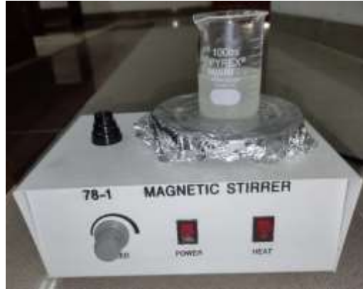
Figure 3.12: Epoxy stirring on magnetic stirrer
