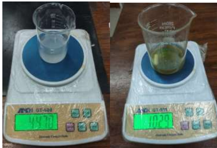
Figure 3.11: Weight measurement for epoxy and hardener
