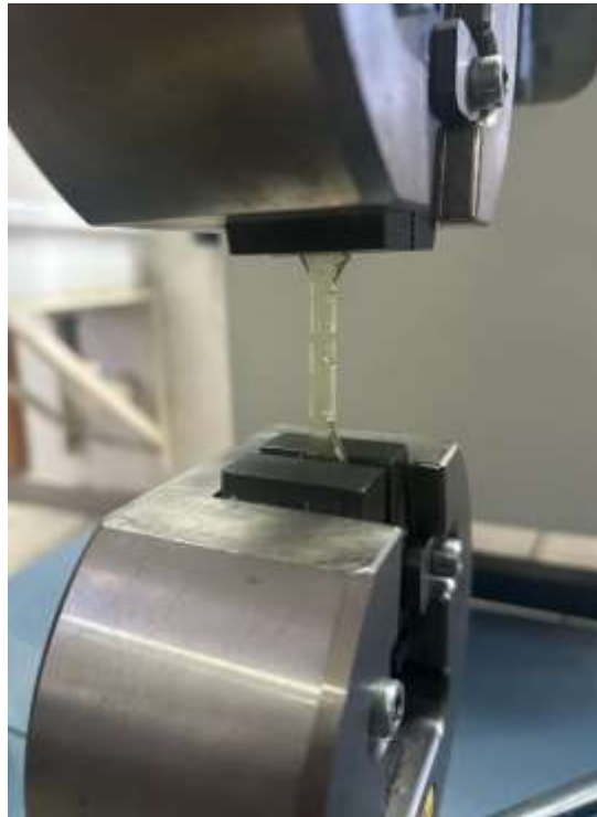
Figure 3.26: UTM testing of Adhesives at Room Temperature
