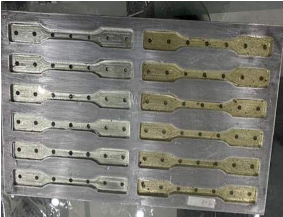
Figure 3.17: Cork powder samples poured inside the mold
