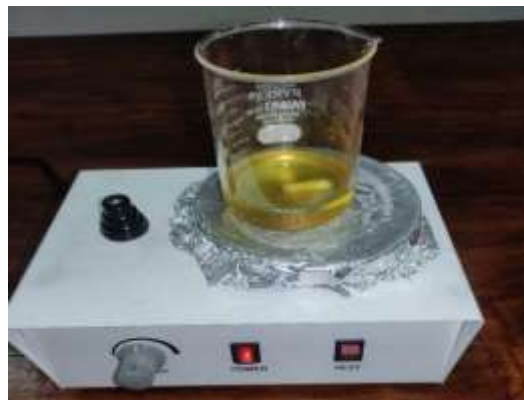
Figure. 3.16 Mixing of hardener
