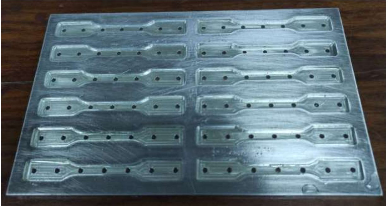
Figure 3.9: Actual Mold made for specimen preparation
