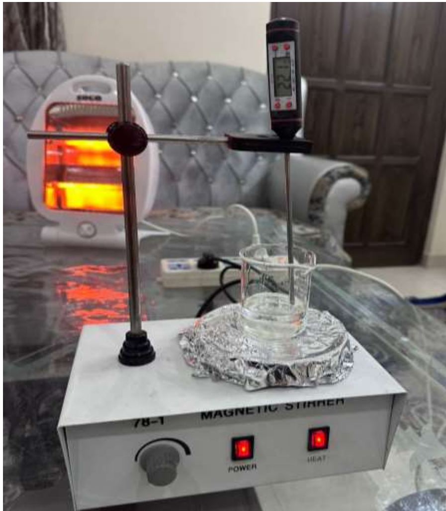
Figure 3.15: High temperature mixing of epoxy and cork powder
