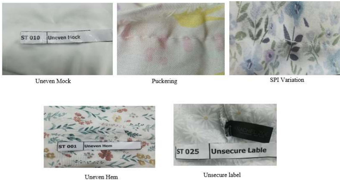
Figure 3.9 Stitching inline defects.
