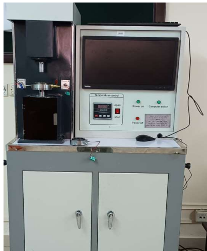
Figure 5.2: Vertical Universal Friction Testing Machine (MMW-1A).
