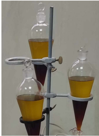
Figure 2.3: Formation of glycerol and impure bio-diesel layer[1].
