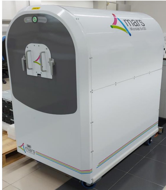
Figure 3.2: Shows the MARS Microlab 5x120, a cutting-edge spectral photon-counting CT scanner engineered by MARS Bioimaging Ltd.
