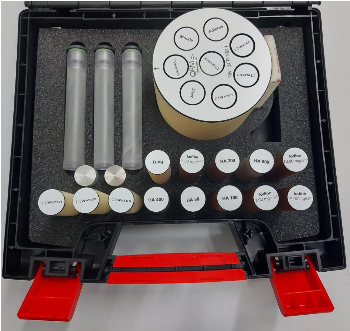
Figure 3.3: Illustrates the QRM Phantom and all the available inserts.
