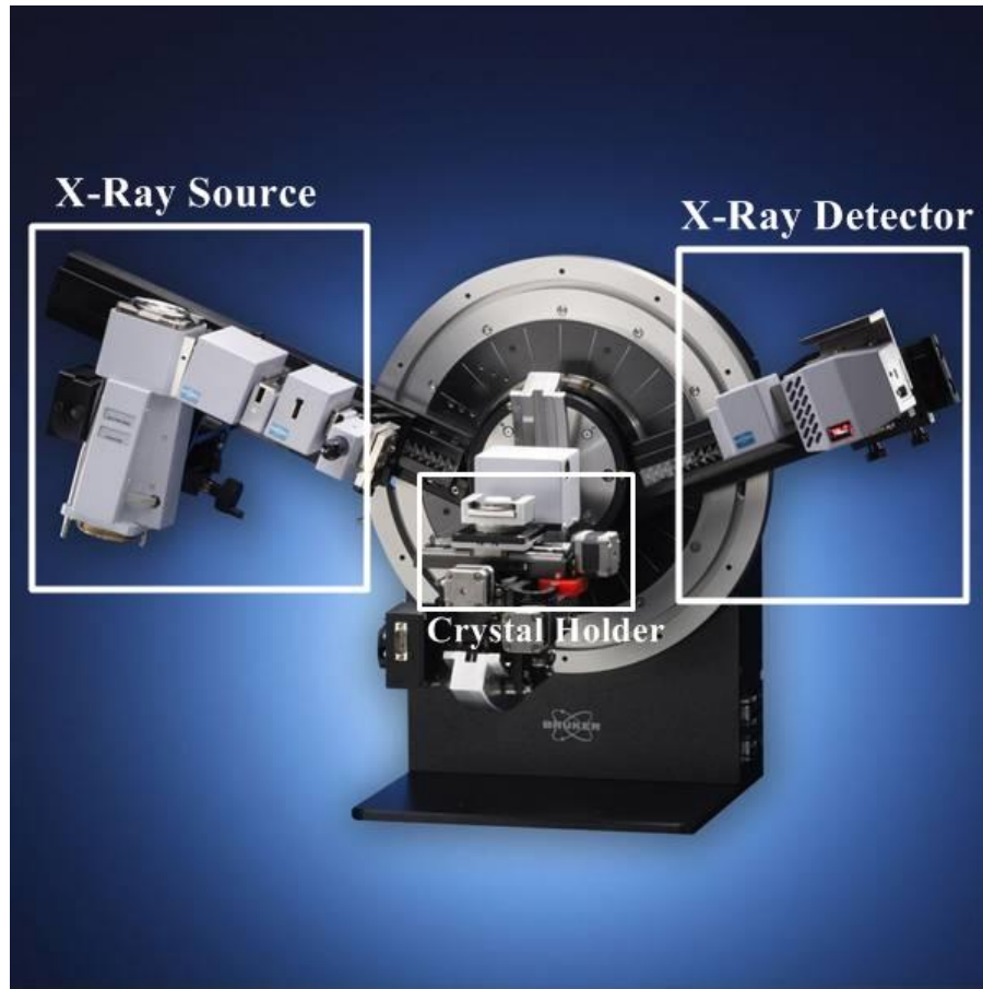
Fig 3.2) Source, sample holder and detector in XRD Machine
