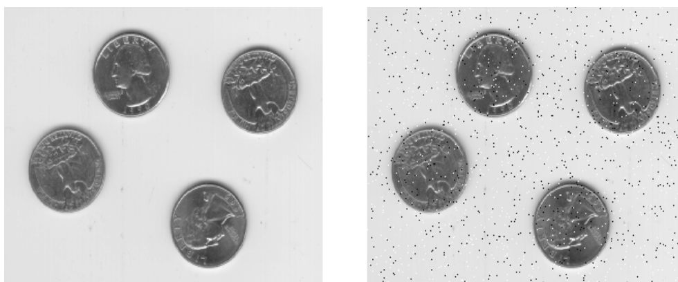
Figure 4.2 (a) Before adding salt and pepper noise (b) After adding salt and pepper noise
