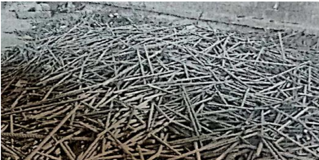
Figure 9 End cut scrap
