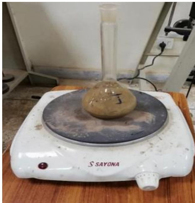
Figure 3.6 Specific gravity test in Progress
