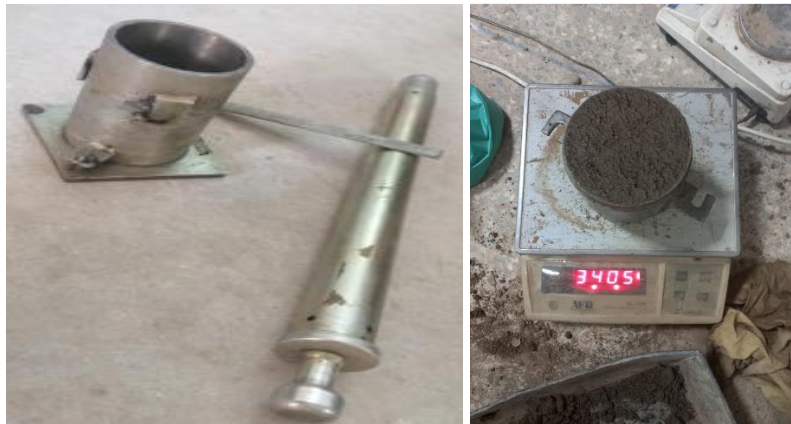
Figure 3.7 Compaction Test Assembly
