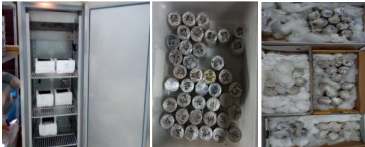
Figure 3.9 Assembly of Freeze Thaw Test
