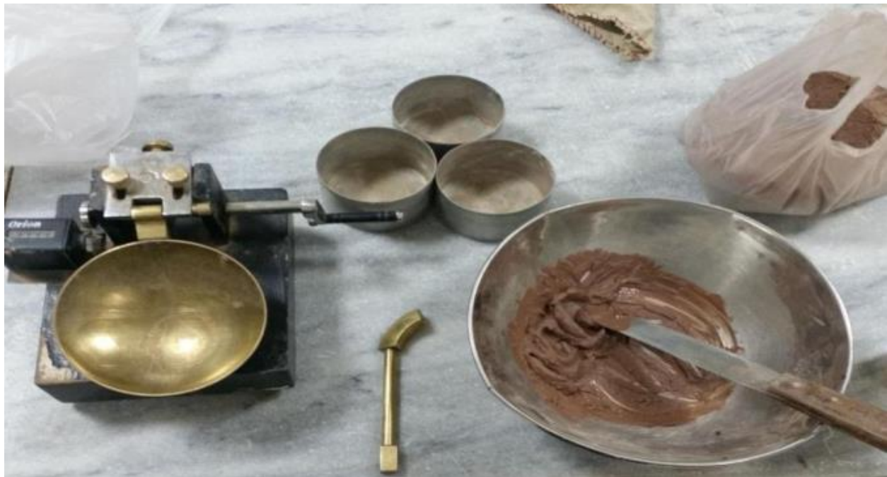
Figure 3.5 Atterberg Limits Test Assembly
