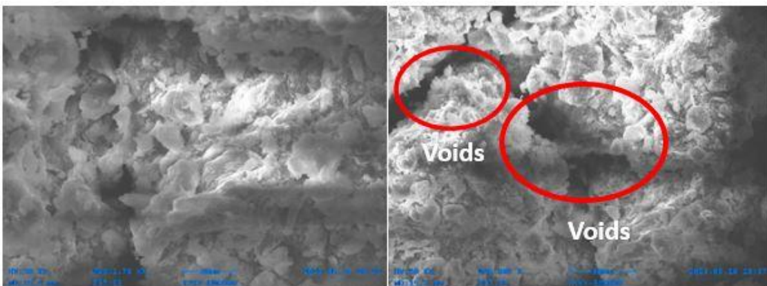
Figure 4.8 SEM analysis of soil B (a) Untreated Sample (b) Untreated Sample under 11 F-T cycles
