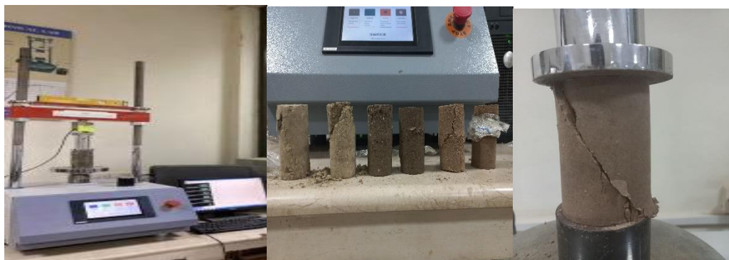
Figure 3.8 Assembly of UCS Test
