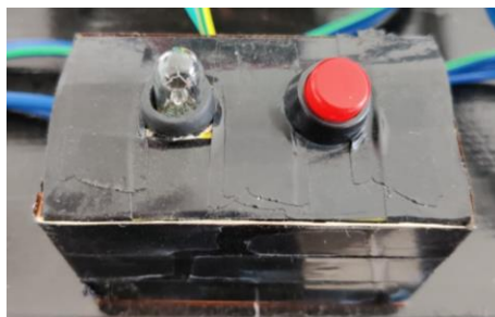
Figure 26 Battery Charging Indicator
