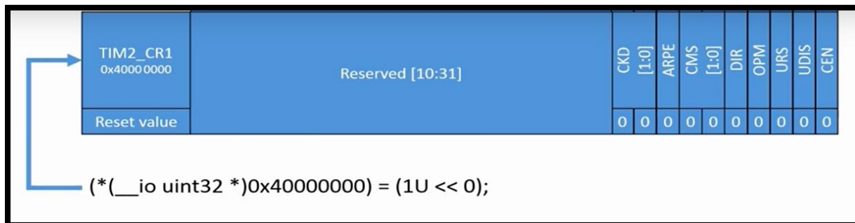
Figure 35: Pointer for Indirect Addressing
