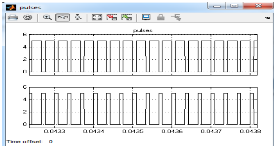
Figure 30: SPWM after comparing both signal
