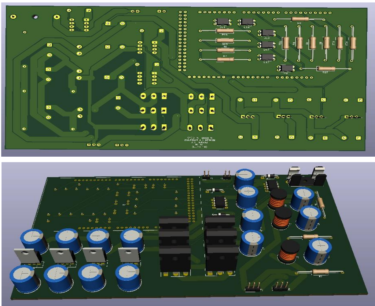
Figure 29: 3D View of PCB
