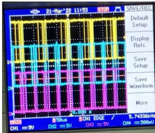
Figure 22: PWM Waveform on Oscilloscope
