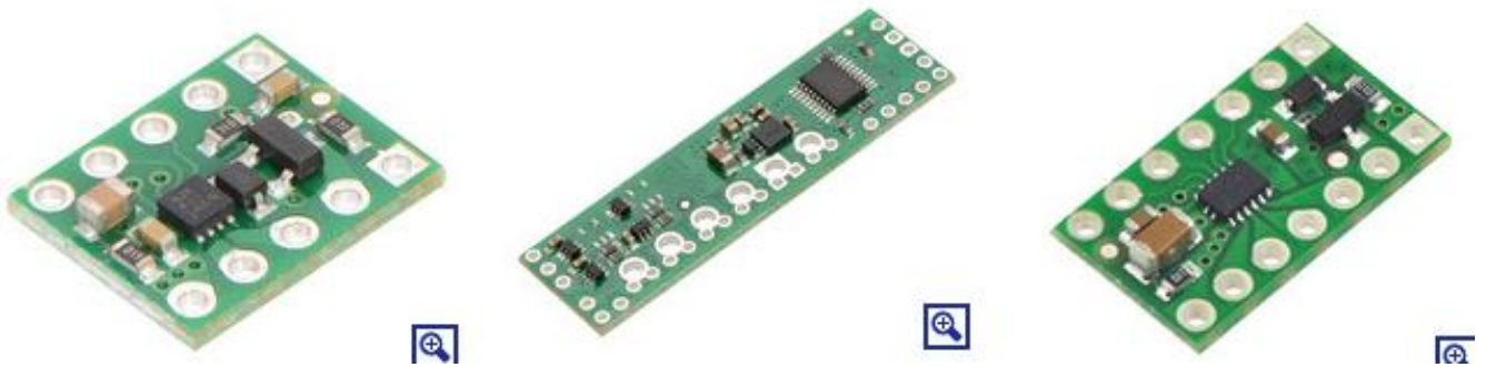
Figure 28: Different types of DC Motor Driver Carriers
