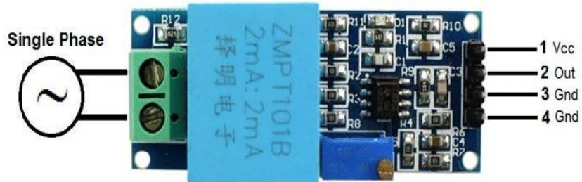
Fig 3.3: Zmpt101B Pin out.
