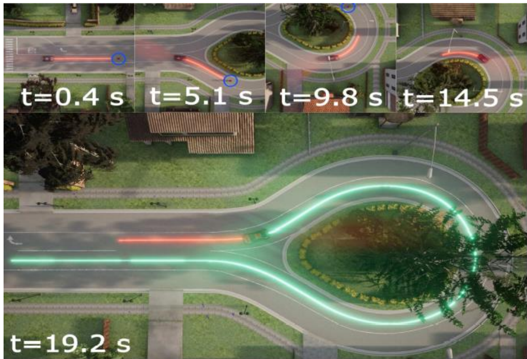
Fig. 21 At various points in time, the trajectory was generated. The effective path taken by the ego-vehicle is shown in green, while the local path planning is shown in red. A blue circle indicates the location of the preceding vehicle (the bicyclist).
