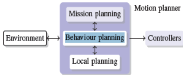
Fig 7. General architecture of motion planning. White boxes denote the scope of the current work.
